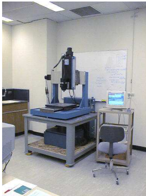
Fig. 10. The MHO 3-axis mill with OpenCNC open-architecture software controller used for the time-optimal feedrate smoothing experiments.
